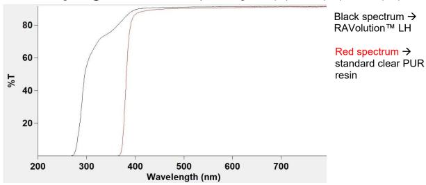
RAVolution™ LH shows a cut off transmittance at roughly 275nm (T%<1.0), while at 315nm where the UV-A radiations band starts, its total transmittance is well above 60%.
