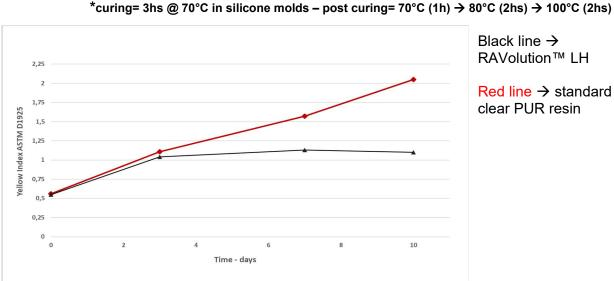
2= Xenon-meter model Q-SUN XE-1-B – 60W/m2 @ 50°C for 240 hs
